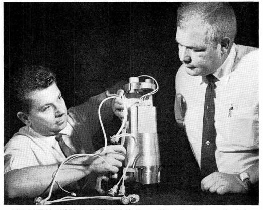
THE SANDIA MILKING MACHINE? Well, no. This telemetry assembly, being checked by Robert Strout (left) and Larry Humphreys (both 8181), was developed by them to monitor about 50 functions during flight test to determine how well system operated. Assembly is used in AEC/DOD programs of post development testing.
